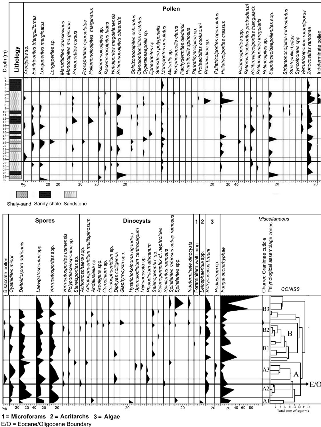
Figure 4b. Palynomorph distribution chart for Olokonla-1 borehole
